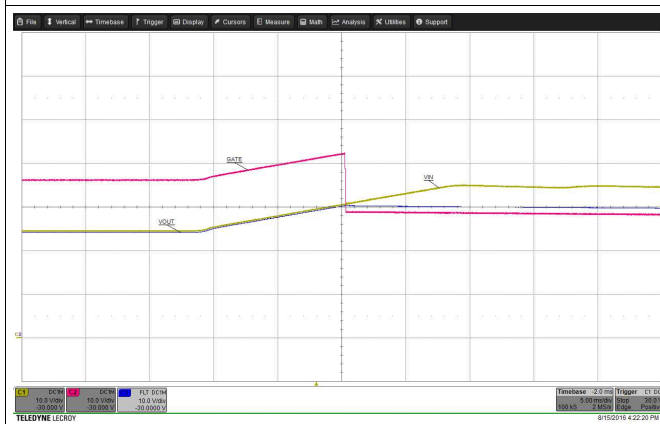
Figure 35. Start-Up into Short Circuit
